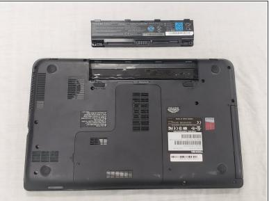
Lifting from the small notch between the two tabs, pull the battery out of the laptop.
