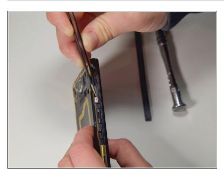
Use the tweezers to remove the pink clips on either side of the device and then take the casing off.
