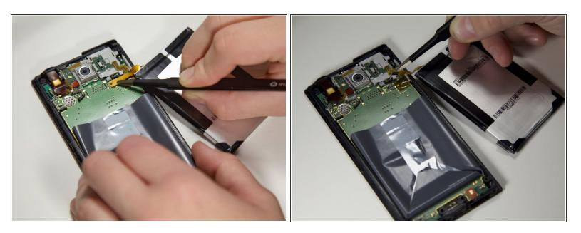
Use the tweezers to remove the Pancake connector that connects the battery to the phone.
