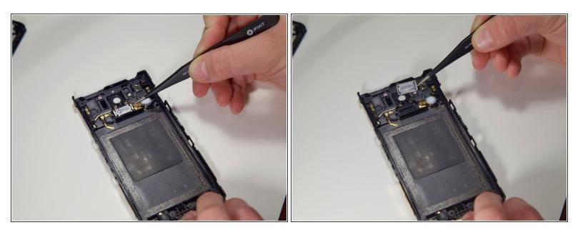
• On the back cover of battery casing, remove the speaker using the tweezers.
