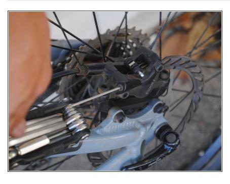
Use a torque spit to remove the indicated screw on the rear brake caliper.
