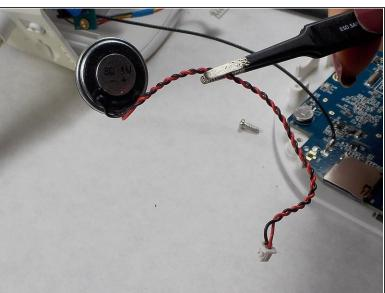
• The speaker is circular, black and silver in color with a red and black cord. It is easily removed from the upper body of the camera with your fingers or safety tweezers.
