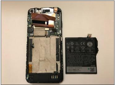
• After prying, simply lift the battery up and out of the device.
