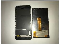
• After the phone is gutted, all that is left is to pry the actual screen off from the backing and prepare for replacement.
