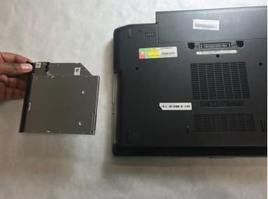
• Grab the spring-loaded tab and pull the drive out from the device.
