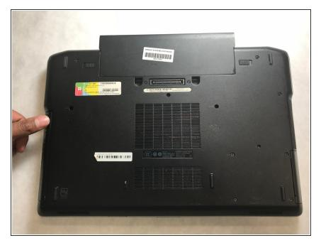
Press open the spring-loaded release tab on the disk drive.
