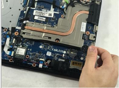
Remove the battery by pushing back the lock with the wedge while pulling the battery up.
