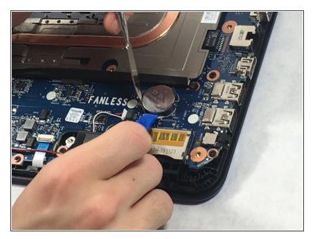
Use a spudger and a plastic opener to push back the lock holding the battery in place.
