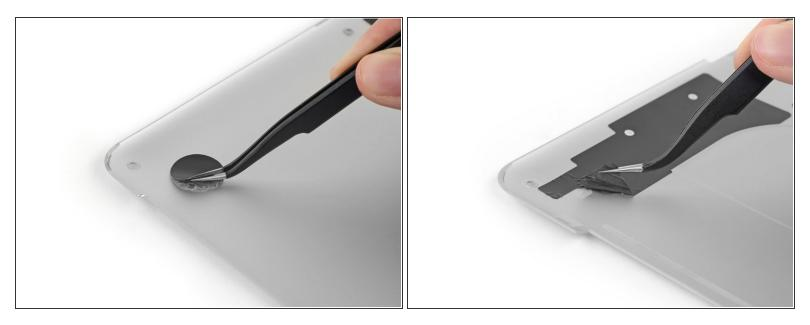
Peel away any stickers from the backside of the rear case covering the feet you have chosen to replace.
