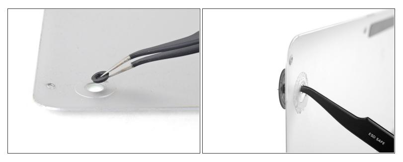
• Remove any broken or damaged feet.
