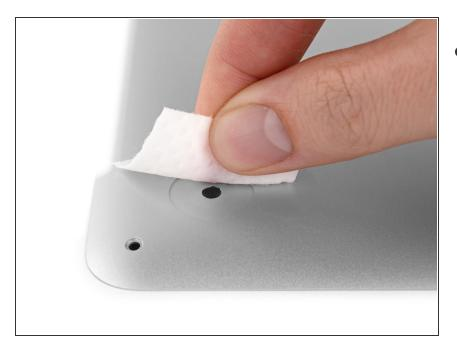
Scrub the foot cavity with adhesive remover to remove any remaining adhesive.
