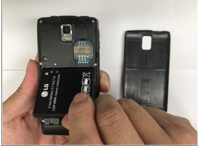
Remove the battery by lifting from the bottom.
