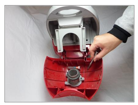
• Unscrew the hose connector from the vacuum cleaner using a Torx 5 screwdriver.
