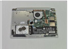
Remove the back panel by pulling it up and away from the laptop.
