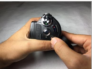
Pull the slider labeled open, on the bottom right, to unlock the battery.
