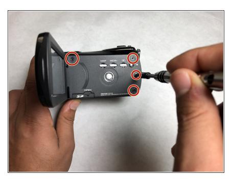
Unscrew the four screws (2.9 mm length) from the screen side of the casing using a JIS000 screwdriver.
