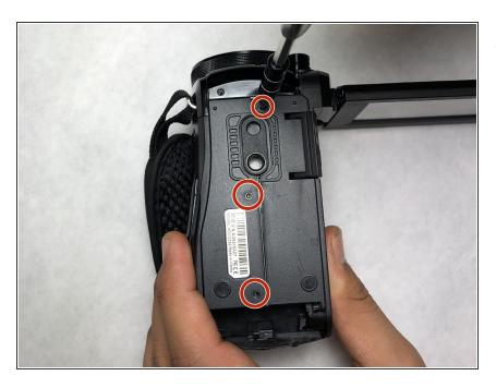
Remove the three screws (length 7.7 mm) from the bottom of the outer case using a JIS000 screwdriver.
