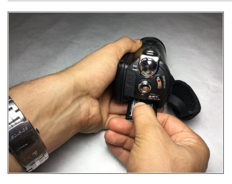
Pull battery out of slot.
