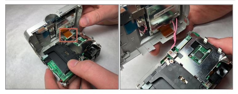
• Remove the orange ribbon cable from its connector by firmly but gently pulling it.
