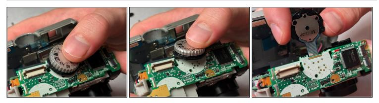
• Push or slide the top dial toward the backside of the camera to unclip from the motherboard.
