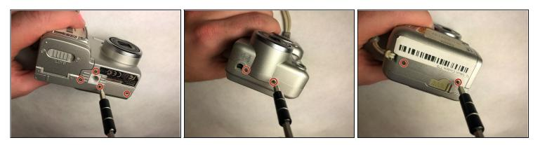
• Unscrew the eight 4mm long JIS #00 screws from the bottom, right side, and the left side.
