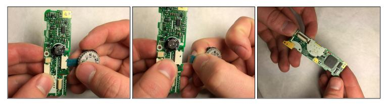
• Pull the ribbon connected to the dial off the motherboard.
