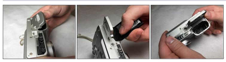
• Flip up the cover and remove the battery inside the slot.
