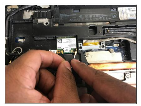
Gently pull the two wires connected to the WLAN Adapter Card.
