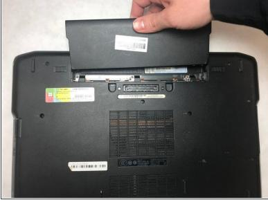
Grasp the battery from the top and pull upward.
