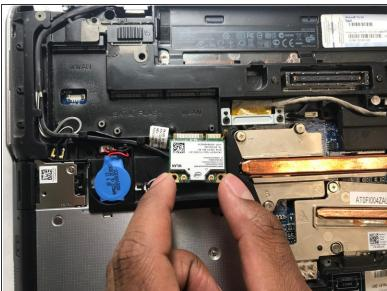
Pull WLAN Adapter Card to remove it from the laptop.
