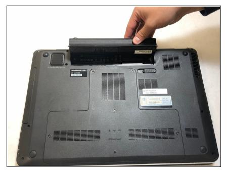
Remove the battery pack from the socket.
