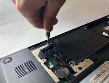
Remove the four 5.7 mm screws, holding down the hard drive, using a Phillips #0 screwdriver.
