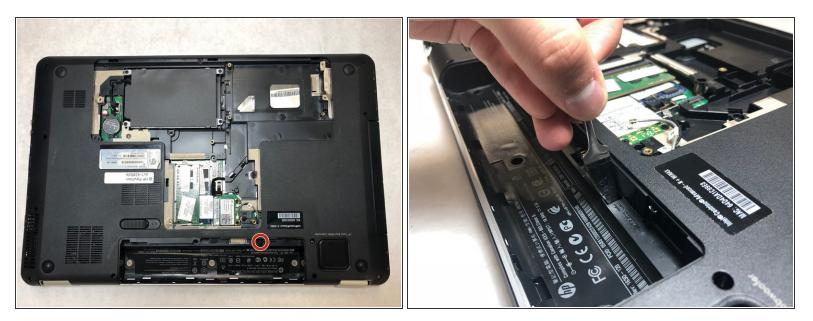
• Push the keyboard release switch using the metal spudger.
