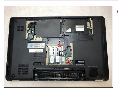
Unscrew the 7.2mm screws using a Ph#0 screwdriver.
