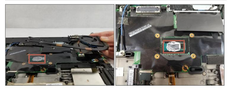
• Lift the fan assembly to gain access to the thermal paste. From here, the thermal paste can be wiped away and replaced. Make sure to only apply new thermal paste to the larger die; don't apply any to the smaller one.
