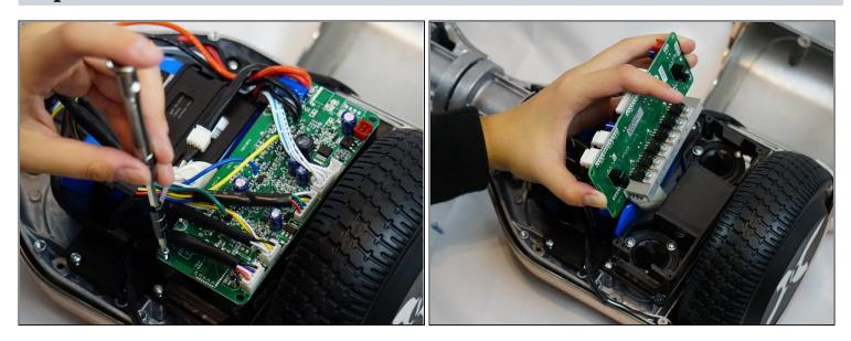
• Locate green electric boards at both ends of the hover board. These green boards are the gyroscopes. Use the screw driver to remove the screws from the corners of the green boards as shown in figure 1.
