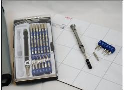
• Locate and use the screw driver and 54 bit as shown in figure 3. Use screw driver to remove screws on the back of the hover board as shown in figure 1. Remove the back shell as shown in figure 2.
