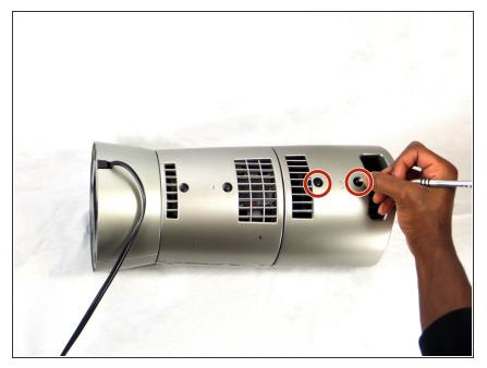
On the backside of the fan, remove the top two 4mm Phillips #Y1 screws using PH 1 bit and Magnetic Driver
