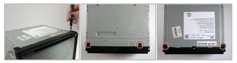
Remove the four 1/8-inch black machine screws using a Phillips #00 screwdriver.
