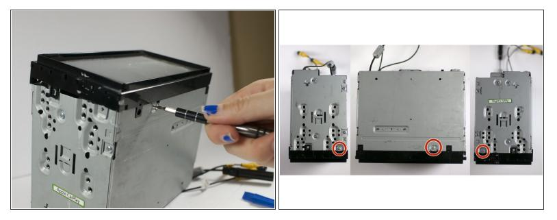
Remove three steel-finish, pan-head, 1/64 x 3/16" machine screws identified in the photograph, using the Phillips #0 screwdriver.
