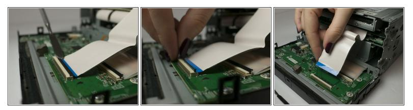
Gently separate the ribbon cable from from ZIF connector on the circuit board using a metal smudger.
