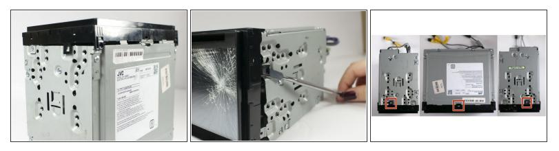
Using your fingers and/or a metal spudger, gently release the plastic locking tabs of the front panel assembly from the steel enclosure while prying the front panel assembly away from the steel enclosure with your fingers.
