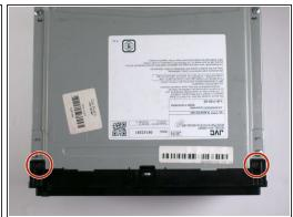
Remove the four 1/8-inch black machine screws using a Phillips #00 screwdriver.
