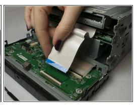
Gently separate the ribbon cable from from ZIF connector on the circuit board using a metal smudger.
