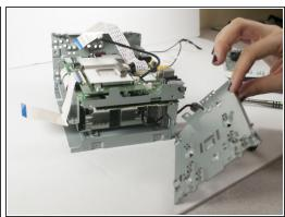
• Remove the five pan-head, 1/64 x 3/16" machine screws using a Phillips #0 screwdriver.
