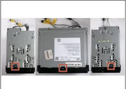
Using your fingers and/or a metal spudger, gently release the plastic locking tabs of the front panel assembly from the steel enclosure while prying the front panel assembly away from the steel enclosure with your fingers.
