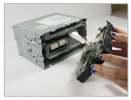
Gently remove the front panel from the steel enclosure.
