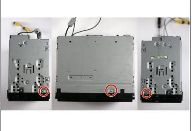
• Remove three steel-finish, pan-head, 1/64 x 3/16" machine screws identified in the photograph, using the Phillips #0 screwdriver.
