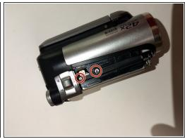
Remove indicated screws to release back panel.
