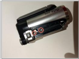
Remove indicated screws to release back panel.
