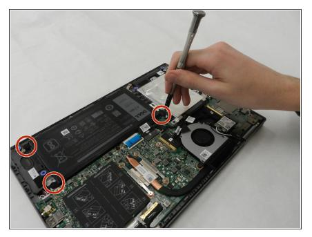
Use a Phillips #0 screwdriver to remove the three 3 mm screws holding the battery in place.
