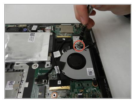
Use a Phillips #0 screwdriver to remove the 3mm screw and the metal bracket that holds the network adapter card in place.
