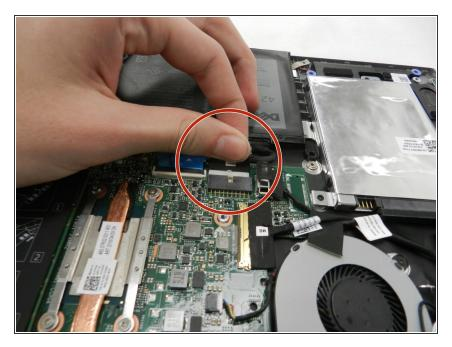
Disconnect the cable connecting the battery to the motherboard, and then remove the battery
