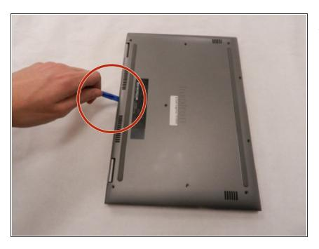
Use a prying tool to remove the back plate.
