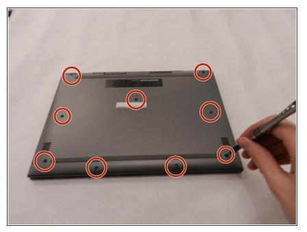
Use a Phillips #0 screwdriver to remove the 9.6 mm screws securing the back plate of the laptop.
