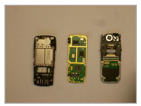
The circuit board should be divided into three parts, completely separate from the back casing, as shown.
