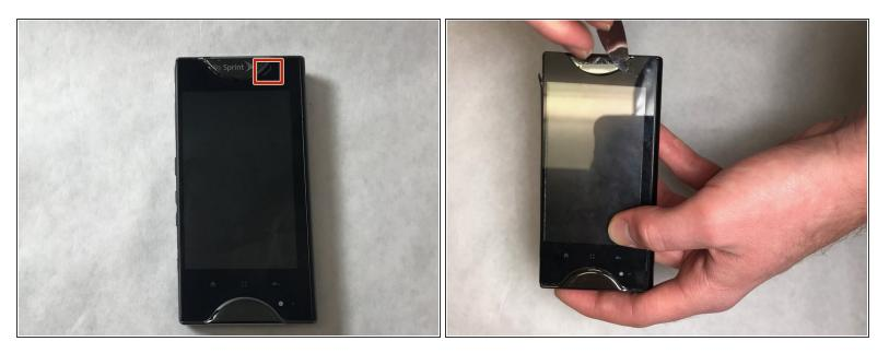
Orient the phone so that the screen is facing up. Place the metal spudger in the half-circle opening located near the bottom right of the Sprint logo at the top of the screen, identified with a red square.
