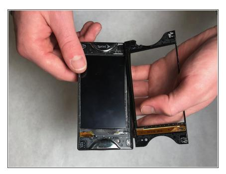
Gently wedge the metal spudger between the top screen and the phone to separate it. Continue wedging along the outside of the screen carefully with the metal spudger until the screen is apart.
