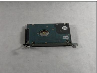
Pull the hard drive out of the hook and remove it from the device.
