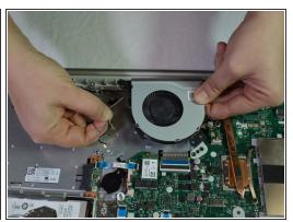
Lift the fan slightly and straight upward and unwind the black and grey wires from the fan.
