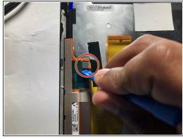
Use the plastic pry tool to remove both of the connections.
