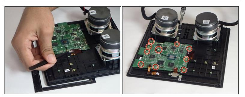
• Unscrew the ten 1mm T5 Torx screws holding the motherboard in place.
