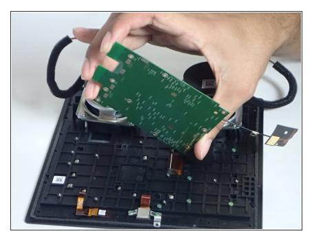
Once all the screws have been removed, you should be able to gently lift the motherboard up and out of the device.
