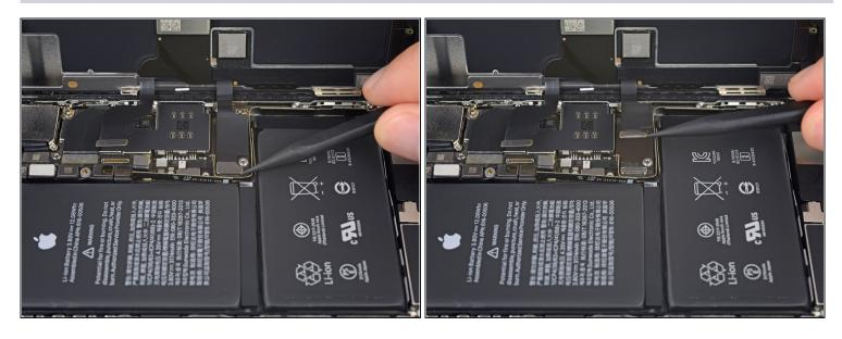
Use a spudger or fingernail to pry the digitizer cable connector up from its socket.
