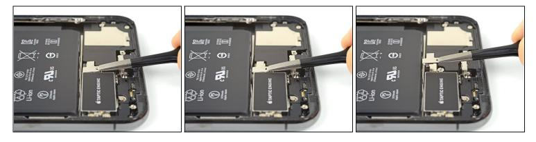
• Push the speaker connector cover towards the battery, and then lift to unclip and remove it.
