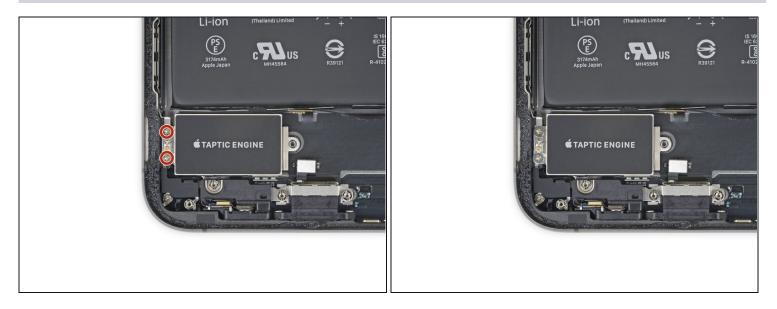
• Remove the two 1.9 mm Phillips screws securing the Taptic Engine.
