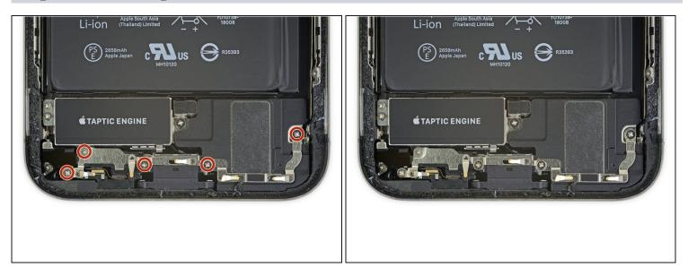
• Remove the five 1.4 mm tri-point Y000 screws securing the bracket below the Taptic Engine and main speaker.
