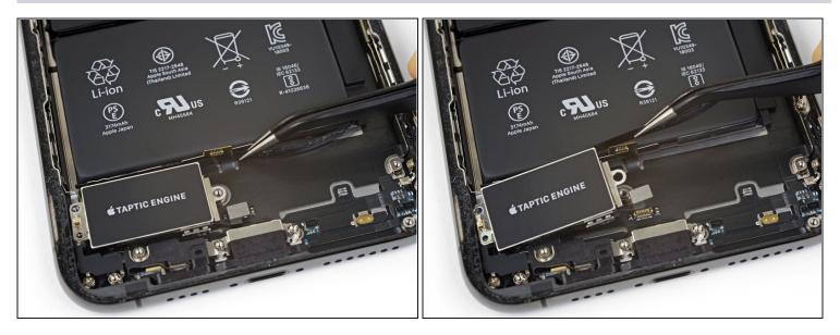
• Grasp the plastic bumper strip and carefully lift it over the speaker connector.
