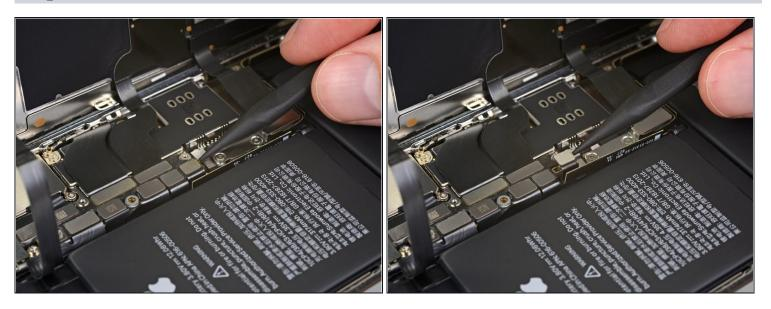
• Use a spudger or a clean fingernail to pry the battery connector up from its socket on the logic board.
