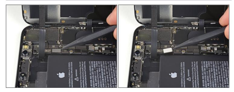
• Use the point of a spudger or a fingernail to disconnect the front panel sensor assembly connector.
