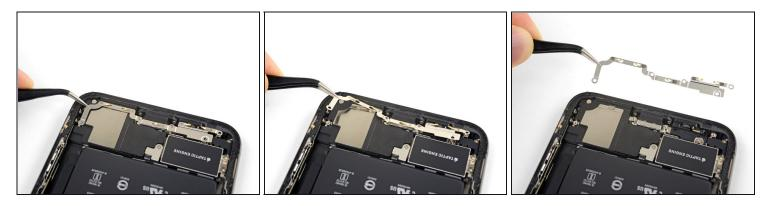
(i) The bracket is lightly adhered in place.
