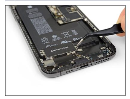
Remove the Taptic Engine assembly.
