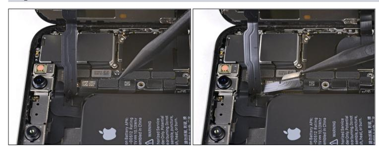
• Use a spudger or a fingernail to pry up and disconnect the front panel sensor assembly connector.
