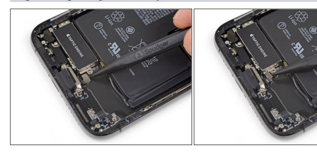
• Use a spudger to disconnect the Taptic Engine flex cable by prying it straight up from its socket.
