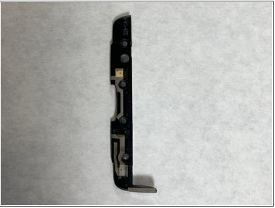
Once the screws are removed, use a plastic spudger and lift up the two plastic pieces that were secured by the screws.
