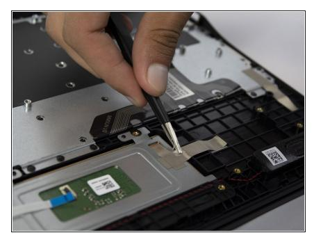
• Using tweezers, remove the silver electrical tape.
