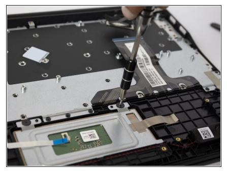
• Using the Phillips Head Screwdriver, remove the screws at the topmost part of the panel holding the trackpad in place.
