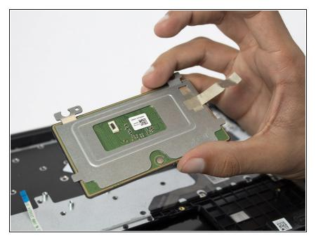
• Carefully remove the trackpad from the computer.
