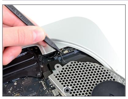
Use the tip of a spudger to carefully pry the antenna connector up from its socket on the AirPort/Bluetooth board.
