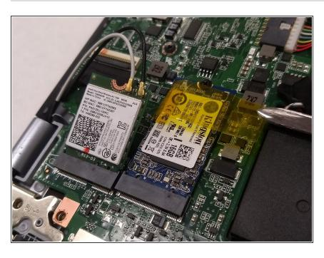
When the screw has been removed, the board will naturally spring up.
