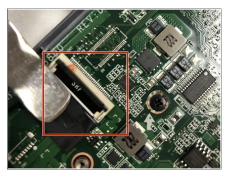
Use metal spudger tool to release the lever that holds the data cable to the board.
