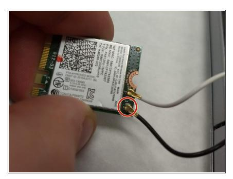
Disconnect the black wire that is plugged onto the 1 or AUX terminal by simply lightly pulling it from the board.
