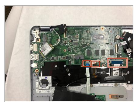
Remove all three cables with a spudger that were hidden by the battery.
