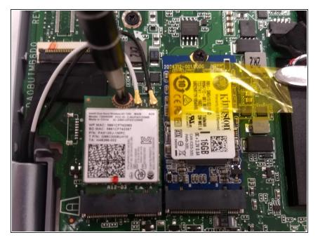
Carefully peel back the yellow tape by either folding it back or removing it entirely. Use the same PH0 Phillips head screwdriver to remove the single screw that connects the motherboard to the Wi-Fi PCB.
