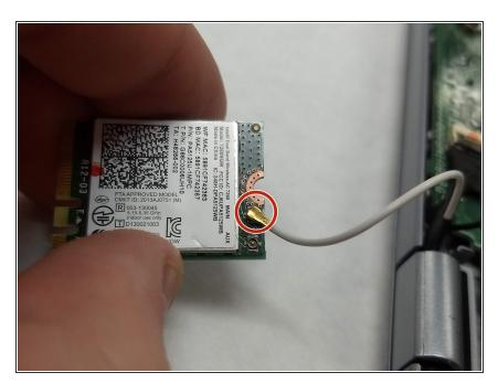
Disconnect the white wire from the 2 or Main plug by lightly pulling it from the PCB.
