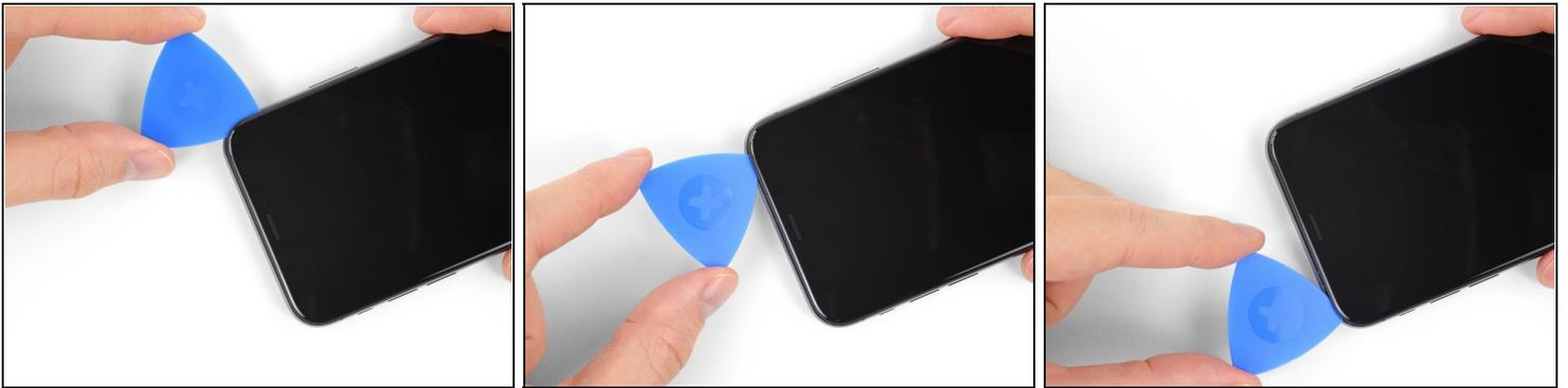
① The top edge of the display is secured with both glue and clips.
