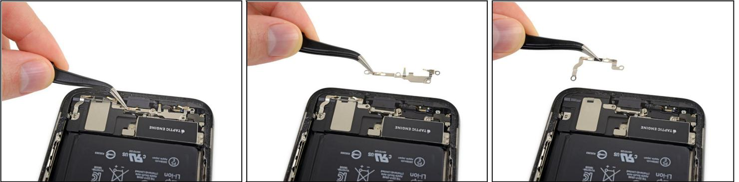
ⓘ The brackets are lightly adhered in place.
