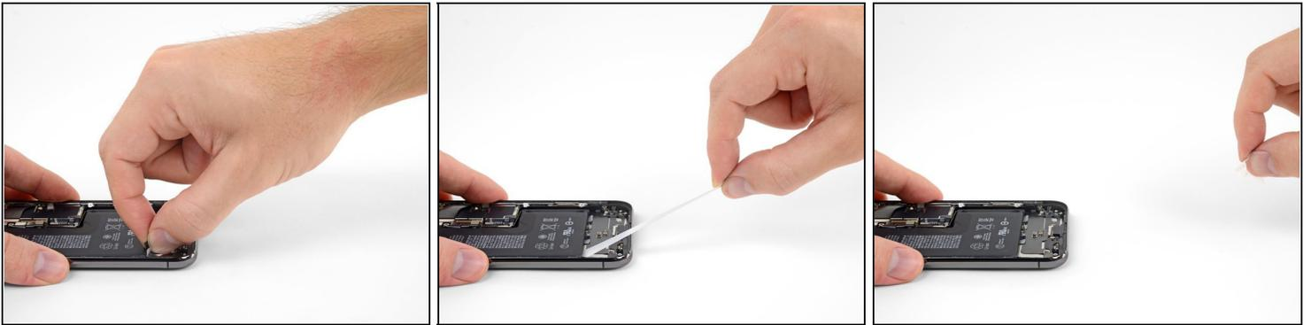
ⓘ In the following steps, you'll pull each tab to slowly stretch out the adhesive underneath the battery. This special stretch-release adhesive loses its tack when stretched and then comes out in your hand, allowing you to lift out the battery with ease.
