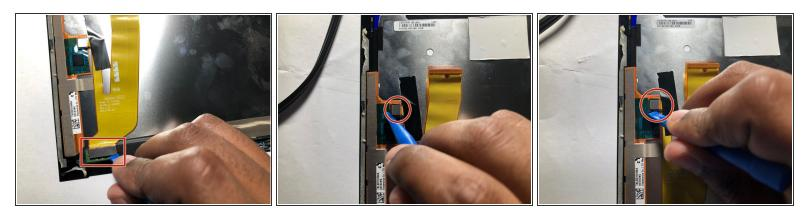
• Use the plastic pry tool to remove both of the connections.
