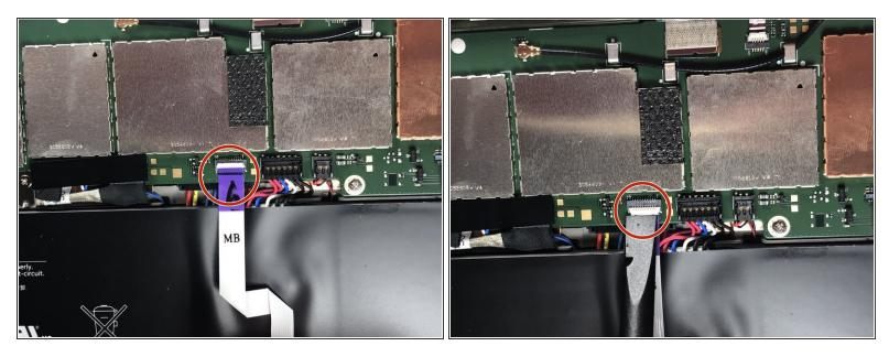
• Remove the ribbon located over the battery.
