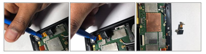
• Take the pry tool and remove the ribbon cable from the logic board.
