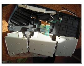
Use the tip of a spudger to push the upper button assembly buttons out from the back.
