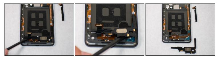
• Use a plastic spudger to pry the loudspeaker out of its recess in the case.
