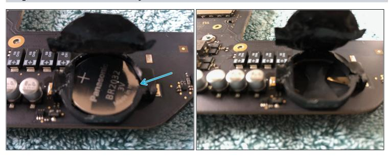
• Use a spudger or small screwdriver to push the battery to the side and it will flip out
