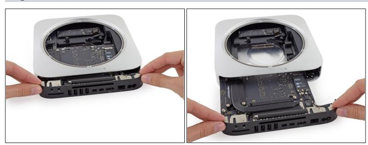
Carefully slide the logic board assembly out of the Mac mini, minding any cables that may get caught.
