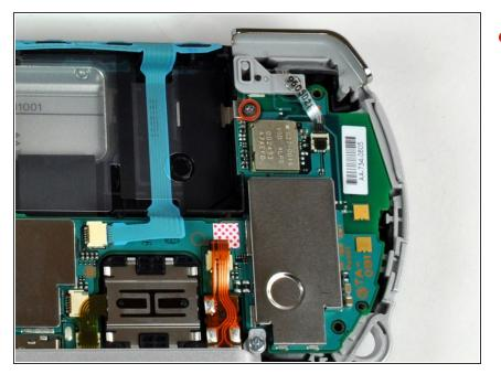
Remove the single Phillips screw securing the logic board to the inner case.
