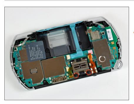
Remove both headphone jack and analog joystick screws using your #00 Phillips screwdriver.
