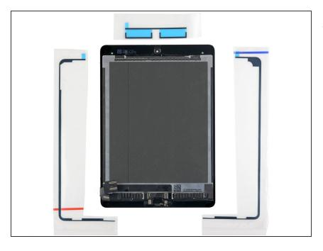
• Lay out the replacement adhesive strips around the display assembly so that they correspond to the correct sides.
