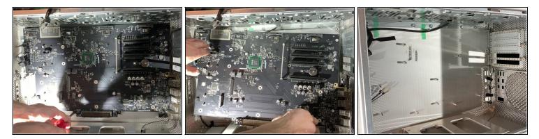
• Unscrew the 10 screws holding in the motherboard
