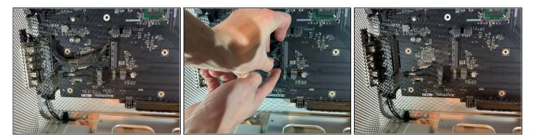
• Remove the ribbon that connects the motherboard to the expansion card (USB, Jack, Power Off etc.)
