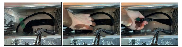
• Push on both knobs to remove the power connector
