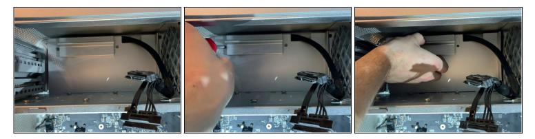
unscrew the two screws and remove the cover
