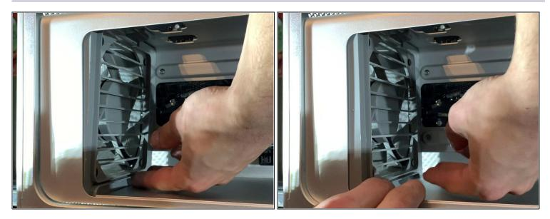
• Similar to the top remove the clip at the bottom and pull out the fan.
