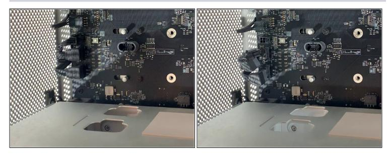
• Behind the fan bracket there are 2 SATA cables, a 4 pin mini power supply and a 4 pin fan
