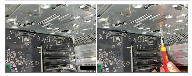
• Unscrew the 4 screws that hold in the power supply
