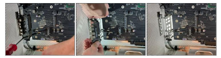
• Unscrew the 6 screws that hold the card in place.
