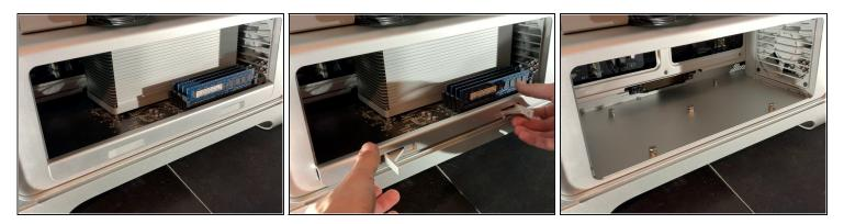
• Press both latches to unlock the bracket and then pull it towards you.
