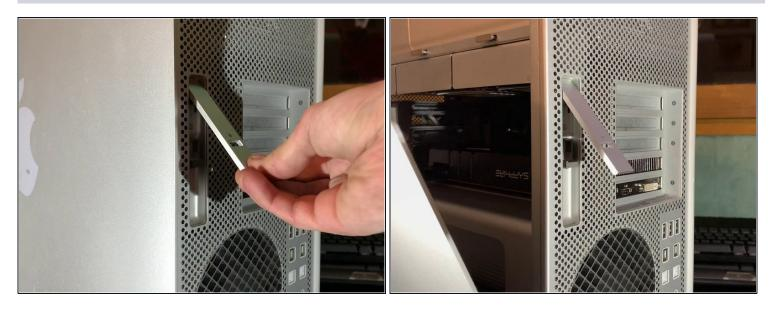
• Lift the flap to put it in the unlocked position, the panel should separate from the box without forcing.
