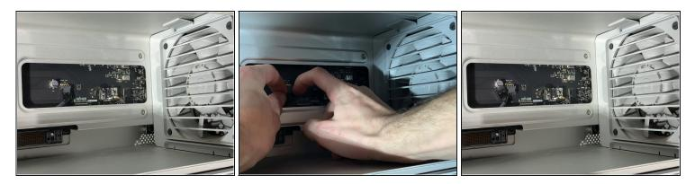
• Disconnect the 2 x 4pin fan cables and the 1 x 2 pin speaker cable
