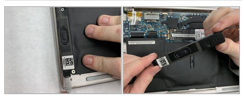
Use a metal spudger or equivalent opening tool to pry and remove the speaker housing from the frame.
