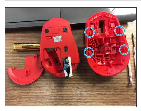
Carefully detach the upper case and the lower case of the mouse by holding the lower case and sliding the upper case forward.
