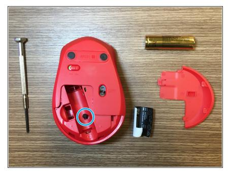
Carefully detach the upper case and the lower case of the mouse by holding the lower case and lifting the upper case up and then pulling it backward.
