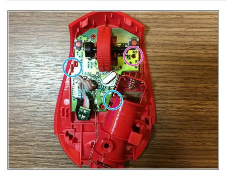
Unscrew the screw in the purple circle and unfasten the plastic pins in blue circles to remove the board from the plastic cover.
