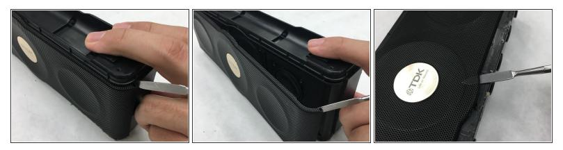
• Use a metal spudger to pry off the front and back mesh screens.
