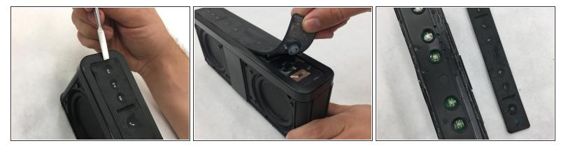
• Turn the speaker back upright. Use the metal spudger to pry up the rubber cover to reveal the buttons underneath.
