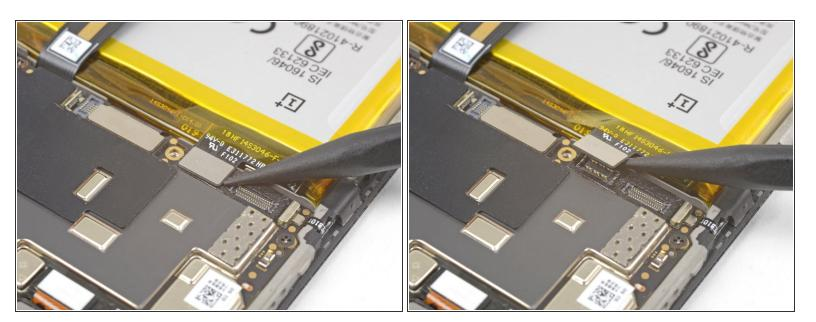
• Use the point of a spudger to pry up and disconnect the battery connector from its socket.
