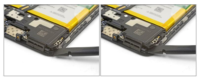
Insert the flat end of a spudger into the corner of the loudspeaker assembly and pry slightly, loosening the loudspeaker from its recess.
