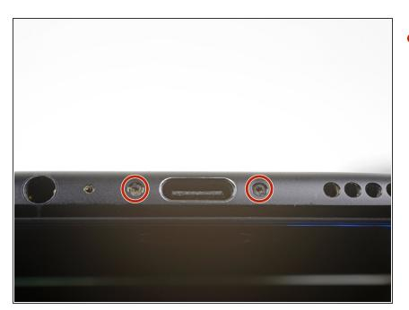
Remove the two 2.6 mm T2 screws straddling the USB-C port on the bottom edge of the phone.
