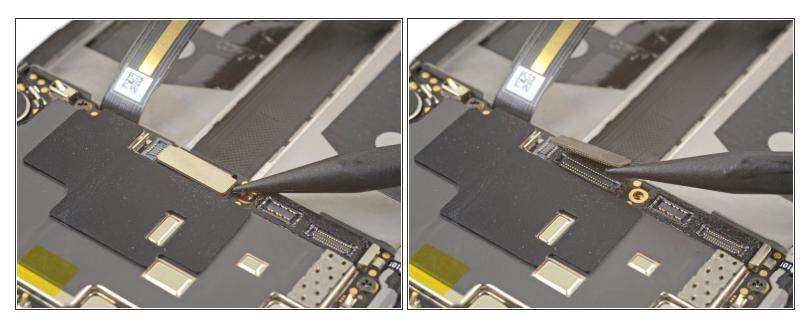
• Use the point of a spudger to pry up and disconnect the display interconnect cable from its socket near the bottom edge of the motherboard.
